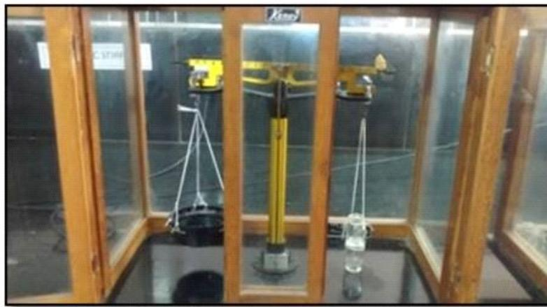
Figure 1: Modified balance for Mucoadhesion study
