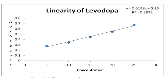
Figure 2: Calibration curve of levodopa (Wavelength maxima at 210 nm of Levodopa)
